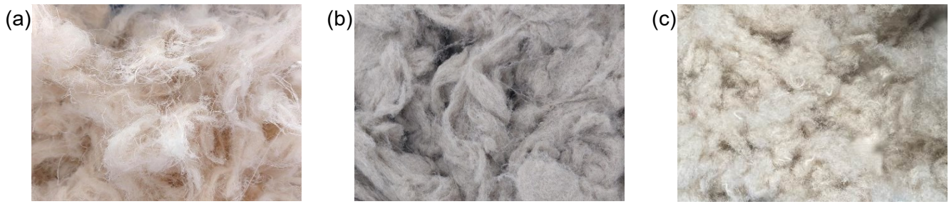
Fig. 1: (a) Hemp 1, German hemp, bleached, not cottonized; (b) Hemp 2, hemp from France, Belgium, Netherlands, unbleached, cottonized; (c) recycled wool from pre-consumer carpets.
