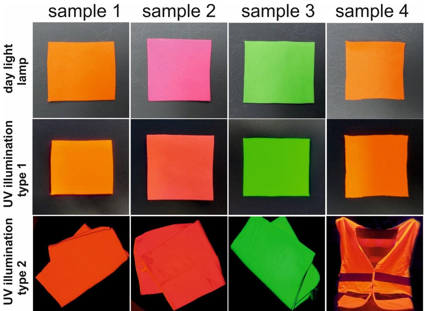
Fig. 2 Overview on different evaluated samples under different kinds of illumination.
