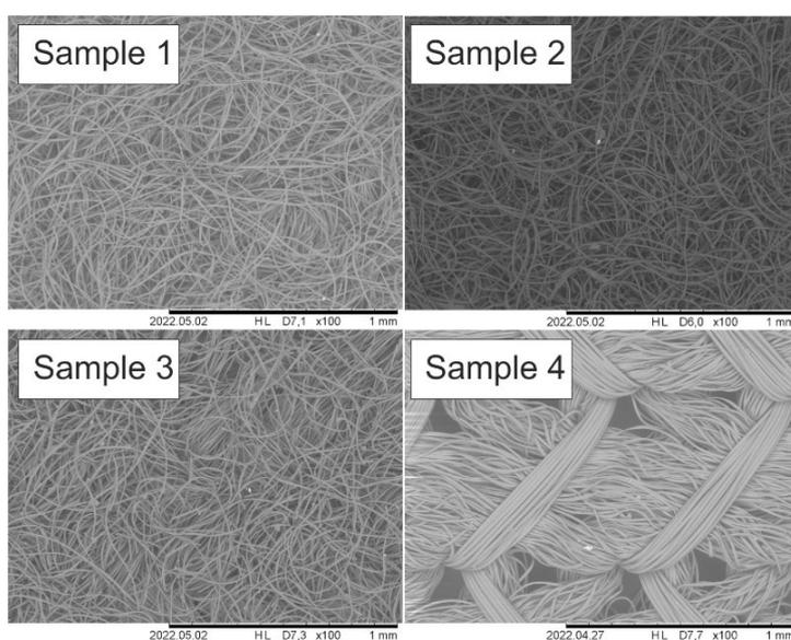
Fig. 1 Microscopic images of the different evaluated samples. These images are recorded by SEM in the same magnification.
