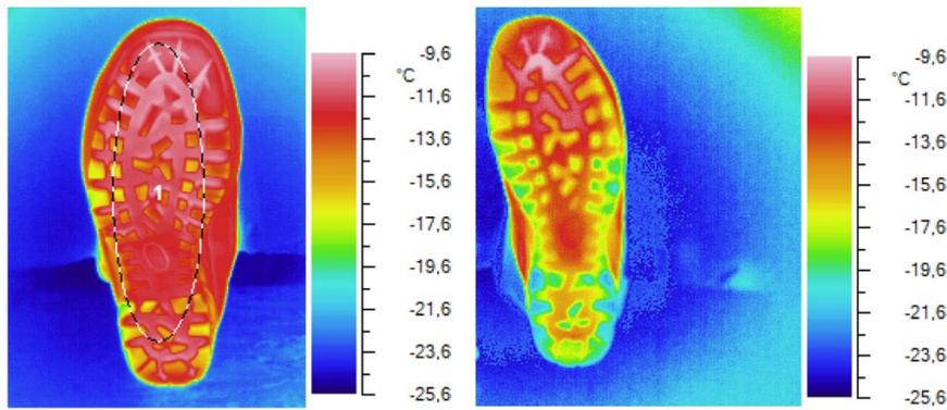
Figure 3. Thermal images acquired at the end of the test for MODEL A (a) and MODEL B (b) both for Tester 1.
