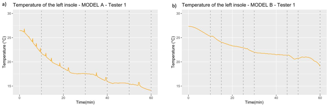
Figure 4. Temperature of the left insole for Tester 1 with MODEL A (a) and MODEL B (b).
