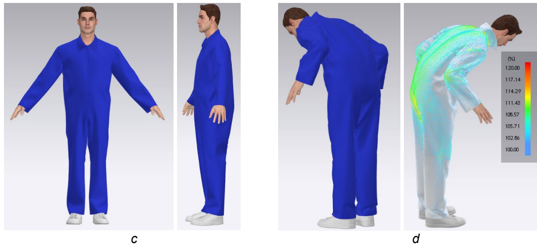
Fig. 6 Newly designed overall: (a) Mathematic relationship for the back length; (b) mathematic relationship for the back width; (c) overall in a static position of the wearer; (d) overall in a dynamic position of the wearer
