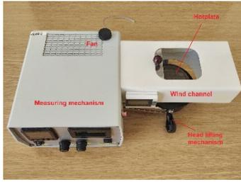
Fig. 3 (a) Permetest skin model in the horizontal orientation
