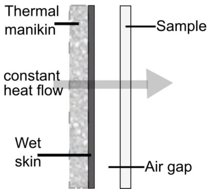
Fig. 1 Principle of thermal manikin
