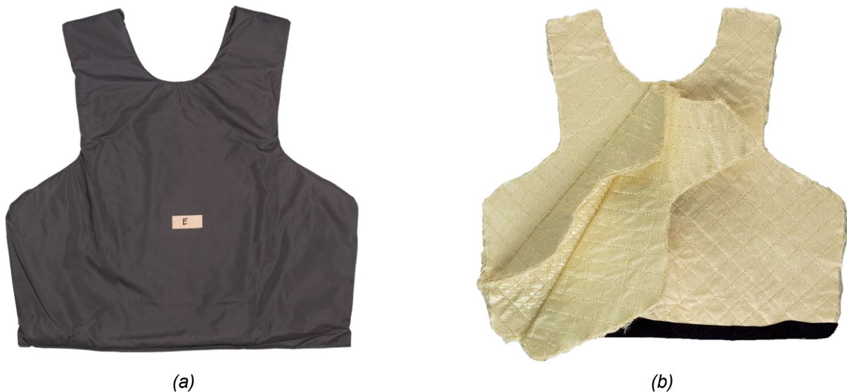
Fig. 2 (a) Multi-layered fabric pack of soft-ballistic vest; (b) 40 layers of aramid woven fabric.
