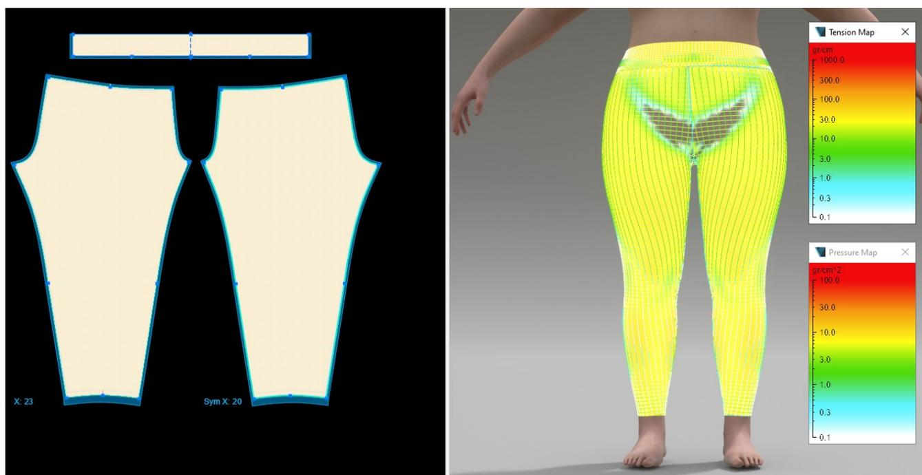
Fig. 1 Legging pattern VStitcher with pressure and tension map.
