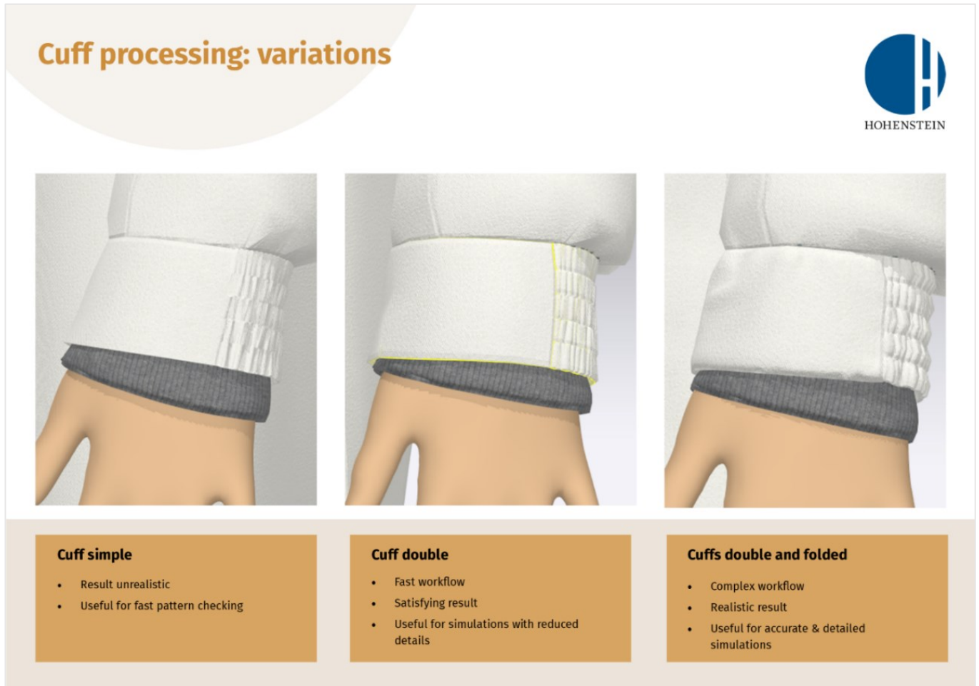
Fig. 3 Extract from the production guideline of a sleeve hem cuff, complex garment winter jacket, CLO3D
