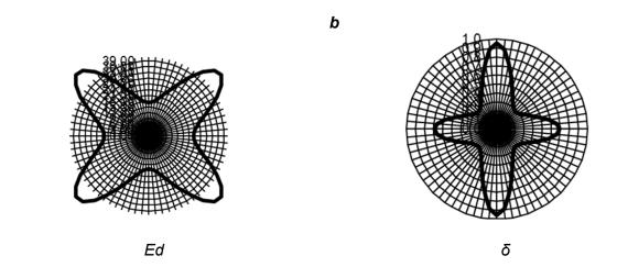
Fig. 7 Diagrams of indicators of (a) the modulus of elasticity Ed (MPa) and (b) the attenuation decrement  $\delta$  of the original materials with duplication parameters Tv.p = 160 °C, Tn.p = 100 °C, t = 15 s.
