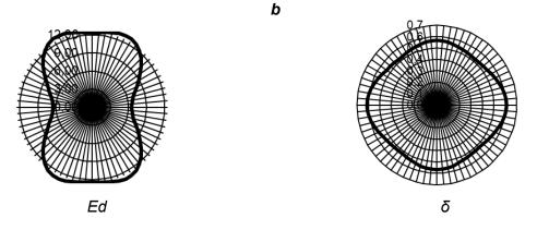
Fig. 6 Diagrams of indicators of (a) the modulus of elasticity Ed (MPa) and (b) the attenuation decrement  $\delta$  of the original materials with duplication parameters Tv.p = 140 °C, Tn.p = 100 °C, t = 15 s.
