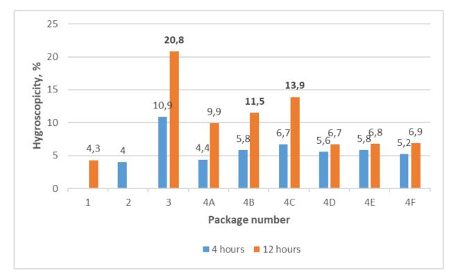
Fig. 8 Hygroscopicity diagram of the tested packaging and original materials
