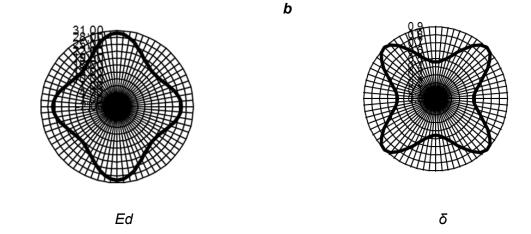
Fig. 3 Diagrams of indicators of (a) the modulus of elasticity Ed (MPa) and (b) the attenuation decrement  $\delta$  of the original materials with the duplication parameters Tv.p = 150 °C, Tn.p = 100 °C, t = 10 s (Tv.p and Tn.p – temperature of the upper and lower pads of the press).
