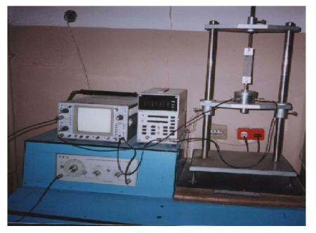
Fig. 1 Installation for determining the dynamic properties of materials.
