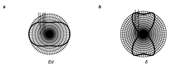
Fig. 5 Diagrams of indicators of (a) the modulus of elasticity Ed (MPa) and (b) the attenuation decrement  $\delta$  of the original materials with duplication parameters Tv.p = 150 °C, Tn.p = 100 °C, t = 20 s.
