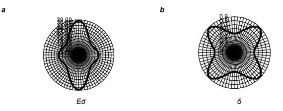
Fig. 4 Diagrams of indicators of (a) the modulus of elasticity Ed (MPa) and (b) the attenuation decrement  $\delta$  of the original materials with duplication parameters Tv.p = 150 °C, Tn.p = 100 °C, t = 15 s.
