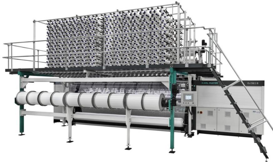
Fig. 2 (a) Example of a stringbar machine
