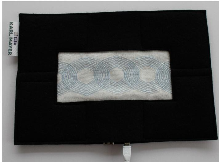
*Fig. 4 Fully textile inductive charging pad*
