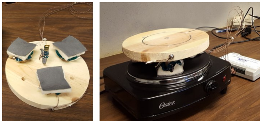
Fig. 4 Apparatus configuration with a heat source at constant temperature.
