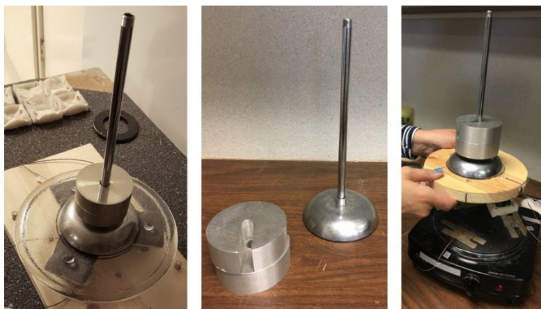
Fig. 5 Method of application of variable weights (center) for two cases of heat sources – cooling heated plate (left) and constant-temperature hot plate (right).
