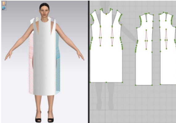
Fig. 8 Simulation in Clo3D (declare seam lines)
