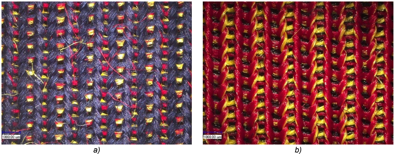
Fig. 2 Microscopic image of the external front taken at a 30x magnification a) on the external front, the estimated values of the sample result in a blue component of 97.3% and a red component of 2.7%. Since none of the front stitches contain yellow, the yellow component is 0%, b) on the external back, the estimated values of the sample result in a red component of 91% and a yellow component of 9%. Since none of the back stitches contain blue, the blue component is 0%.
