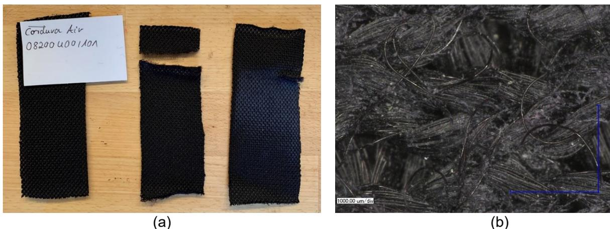
*Fig. 4 Photograph and microscopic image of CORDURA® Air: (4a) reference sample, damaged sample due to the impact simulation and sample after the abrasion test without a fall simulation; (4b) microscopic image of the abraded surface.*
