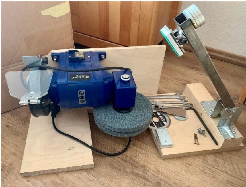
*Fig. 1 A self-built test setup for testing the abrasion resistance of protective clothing.*
