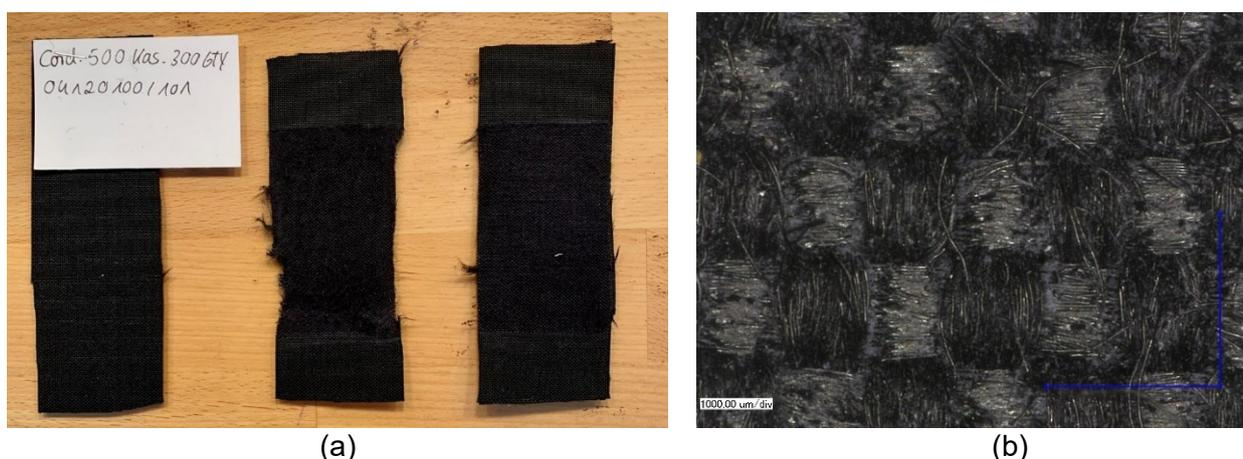
*Fig. 5 The photograph and microscopic image of the CORDURA® 500 (laminated): (a) reference sample, damaged sample due to the impact simulation and sample after the abrasion test without a fall simulation; (b) microscopic image of the abraded surface.*
