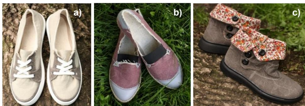
*Fig. 19. Shoe models produced with custom-made last: A – shoes made on the shoe last model 3, B - shoes made on the shoe last model 2, C - shoes made on the shoe last model 1.*
