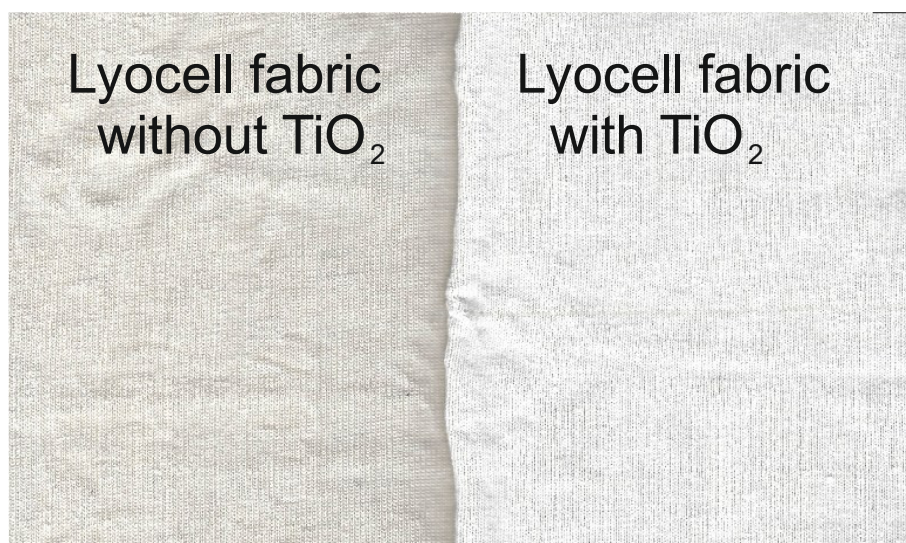
Fig. 3 Color impressions from Lyocell fabrics with and without \text{TiO}_2 additive before application of the dyestuffs.
