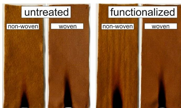
Fig. 9 Bottom-edge ignition test results. Shown are results from untreated Kynol fiber materials (left) and functionalized Kynol fiber materials (right). The functionalization is performed by a combined application of the hydrophobic agent RUCO Dry DHY (125 g/L) and the antistatic agent Zerostat FC NEW (10 g/L).
