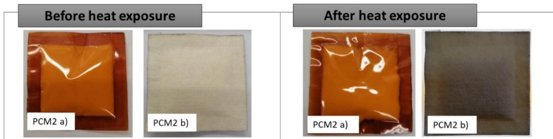
Fig. 6 PCM packages before and after heat exposure: a) film and b) membrane.
