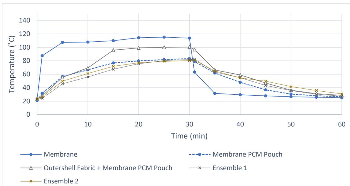
Fig. 9 Thermal performance evaluation of the two ensembles proposed.
