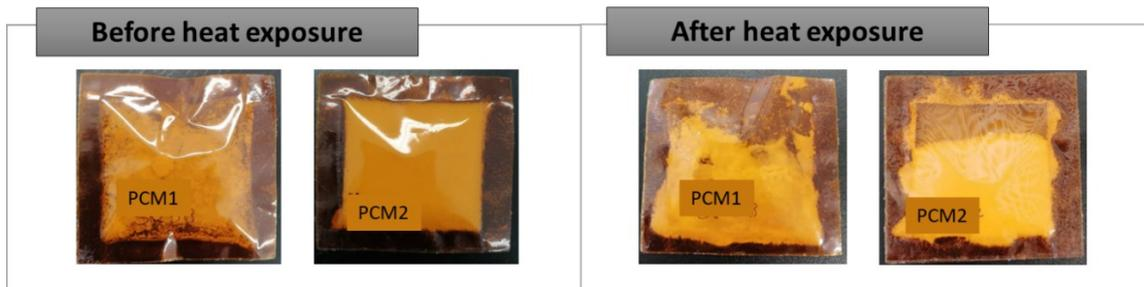
Fig. 5 Film PCM packages before and after heat exposure.
