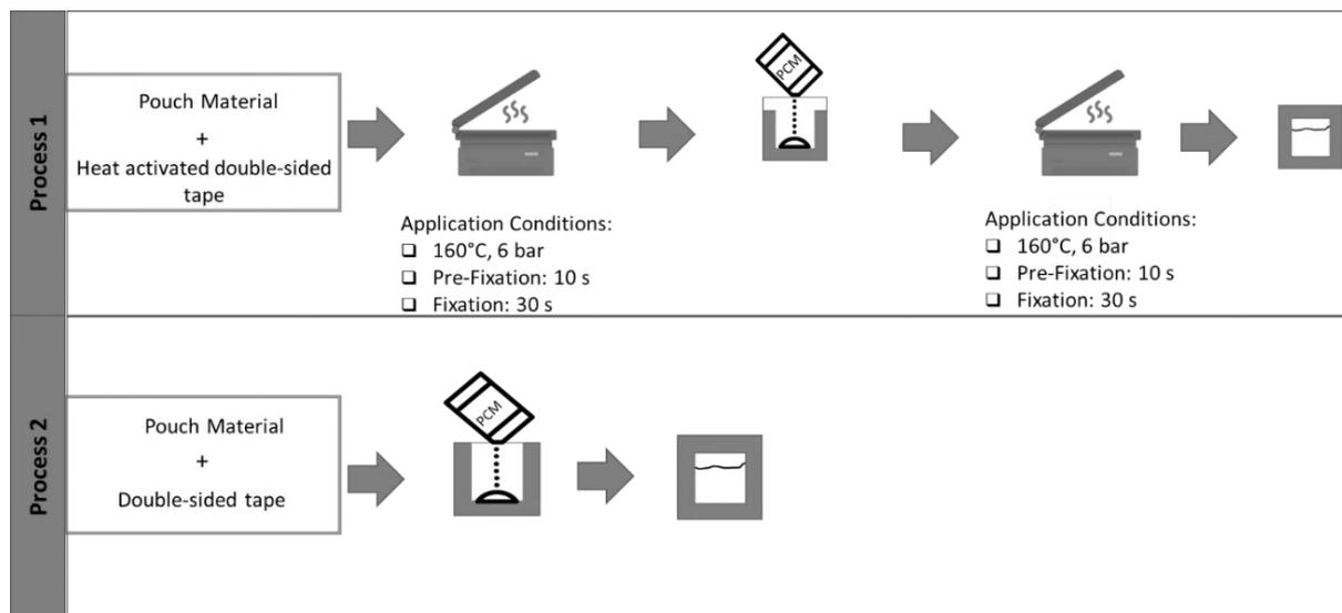
Fig. 2 Different processes used for PCM pouches development using bonding technology.
