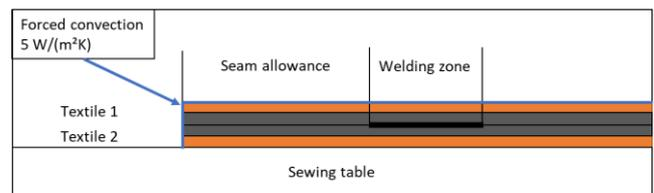
Fig. 12 Thermal sources for numerical calculation around the model “lap seam”.
