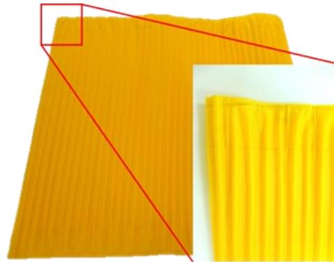
Fig. 5 Ultrasonic-welded temperature control element.
