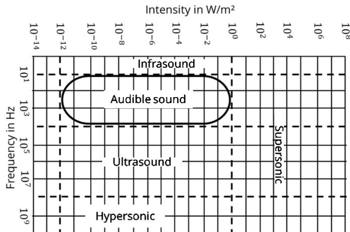
Fig. 8 Classification of mechanical vibrations according to intensity and frequency range [2].
