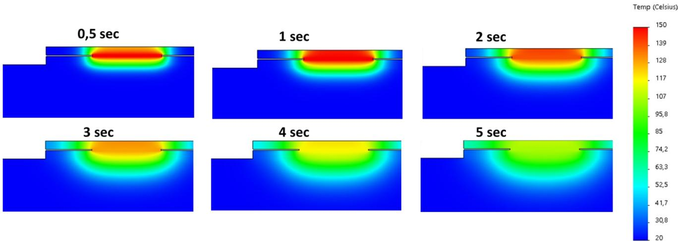
Fig. 15 Transient thermal calculation for a seam spacing of 2 mm.
