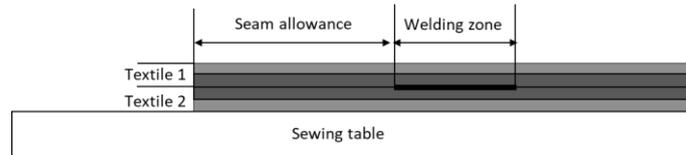
Fig. 10 Model arrangement “Lap seam” for the numerical calculation
