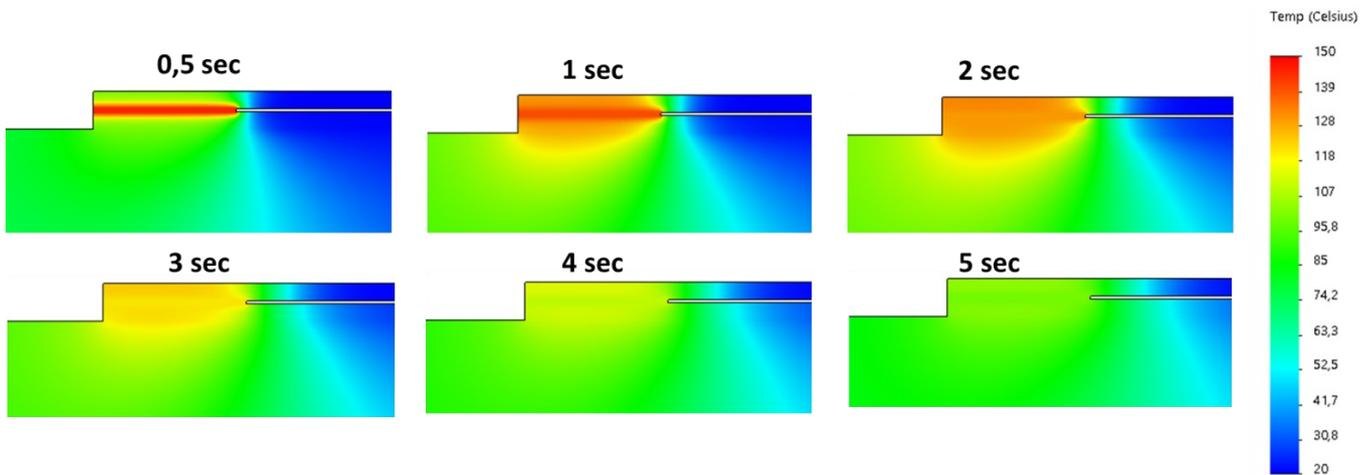
Fig. 13 Transient thermal calculation for a seam spacing of 0 mm.
