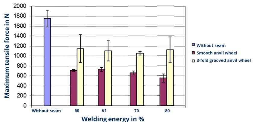
Fig. 3 Maximum tensile forces for different energy inputs and anvil profiles [3].
