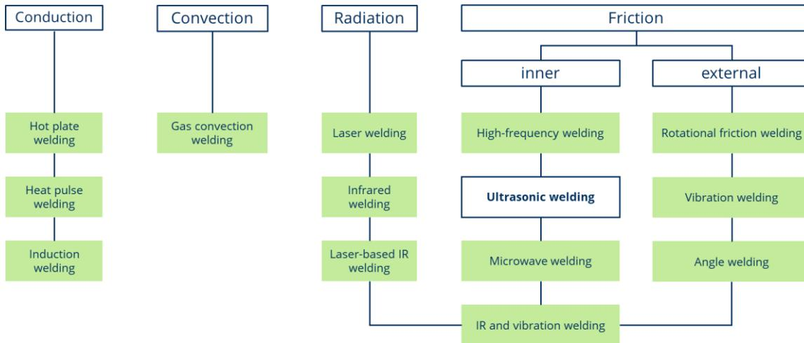
Fig. 1 Classification of welding processes according to ISO 4063 (classification based on type of heat input) [1].
