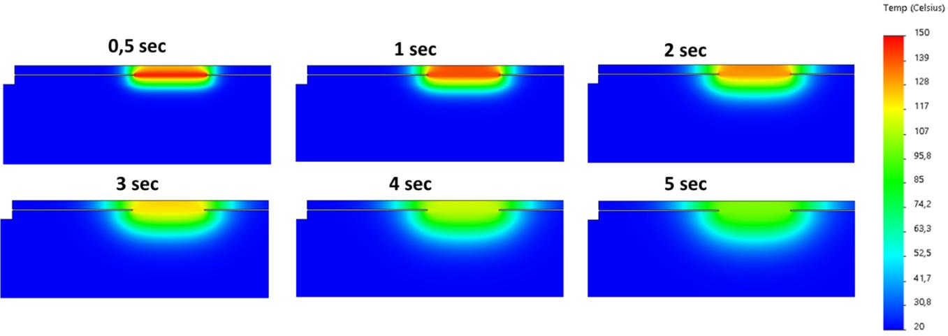
Fig. 16 Transient thermal calculation for a seam spacing of 5 mm.
