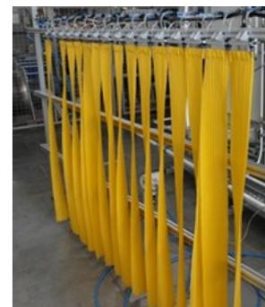
Fig. 7 Textile temperature control element as window curtain [5].
