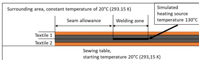
Fig. 11 Thermal sources for numerical calculation in the model “lap seam”.
