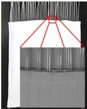
Fig. 4 Tube-based temperature control element.
