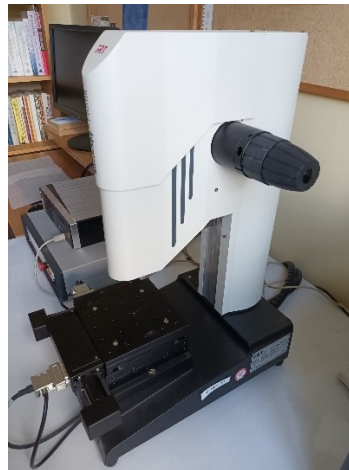
Fig. 3 MicroSpy® Profile profilometer by the FRT the art of metrology™.
