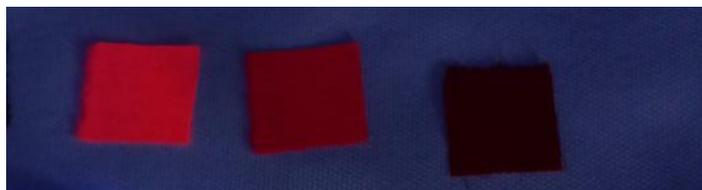
*Fig. 6 Photographs of Rhodamine B containing cotton samples under different illumination (top: daylight; bottom: UV light). The Rhodamine B is applied on the fabrics from a solution containing water and iSys HPX in a ratio 1:1. The dye concentration is increased from left to right (0.5 wt-%; 1 wt-%; 3 wt-%).*
