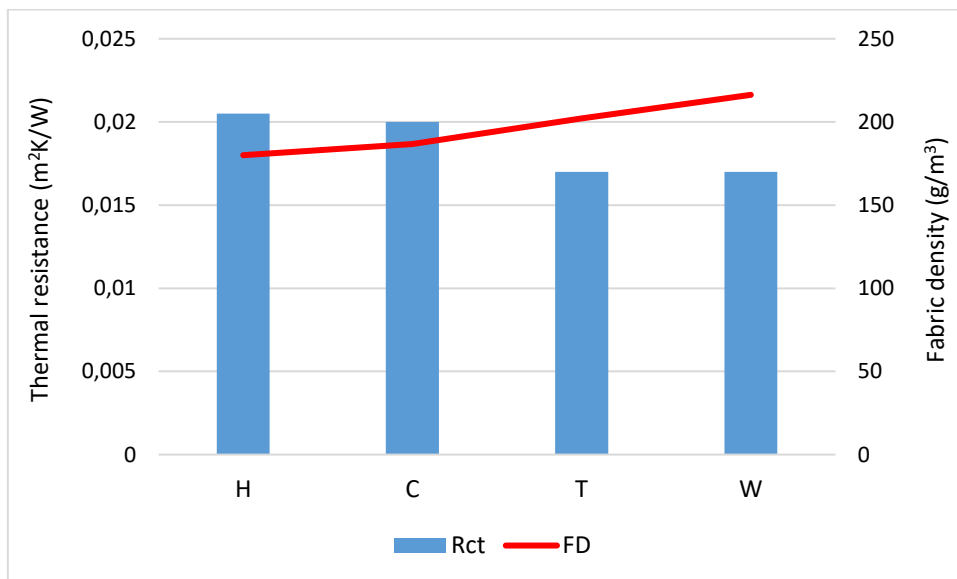
Fig. 7 Relations between the fabric thermal resistance and fabric density.
