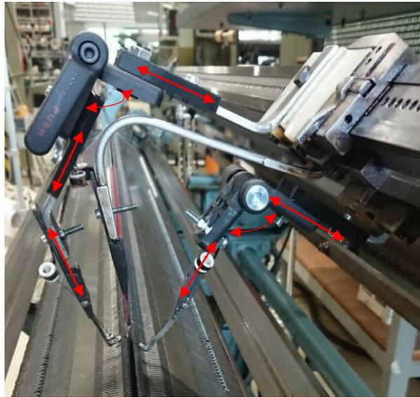
Fig. 6 Attachment of the modular yarn carriers to the knitting machine.
