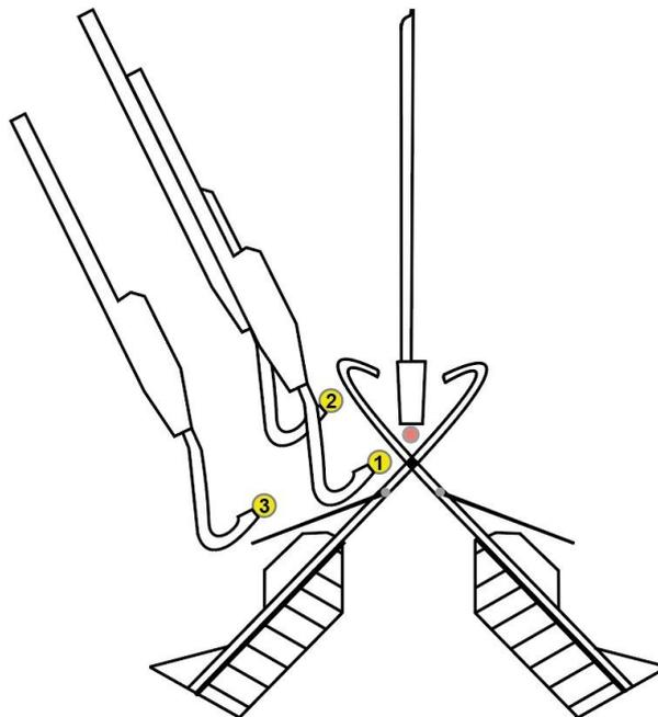
Fig. 8 Yarn carrier 6 is moved into three different positions to find the correct position; adapted from WO2020069856A1.
