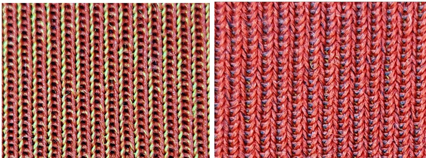
*Figure 10 (a) Back side of the innovative knitted fabric. The red yarn is plated only on one side of the stitch so that the yellow yarn is still visible on the other half; (b) front side of the innovative knitted fabric. The red yarn is plated faultlessly so that the blue yarn is barely visible*
