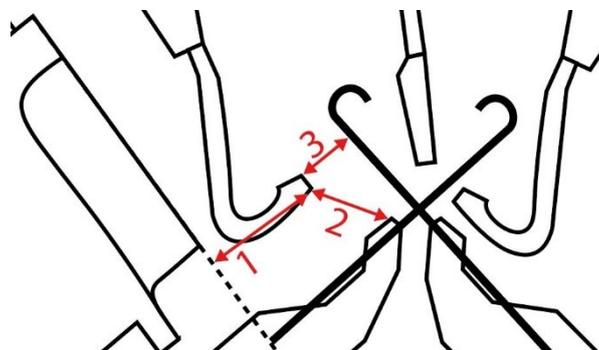
Fig. 7 The three different distances measured to define the exact positions of the yarn carriers.
