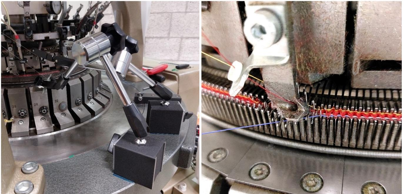
*Figure 9 (a) The yarns F1 and F2 were fed to the needles using magnetic stand; (b) a first yarn F1 is inserted in the cylinder needles. A second yarn F2 is inserted behind the dial needles. A third yarn F3 is inserted into the dial and cylinder needles.*
