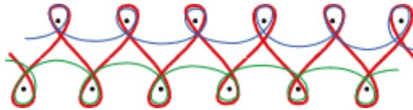
Fig. 4 Needle notation of the innovative knitted fabric.
