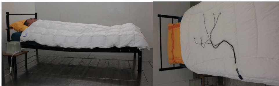
Fig. 2 Measurement setup “Sleeping trial” in climatic chamber with subject (left), position of temperature and humidity sensors (right, duvet turned for visualization).
