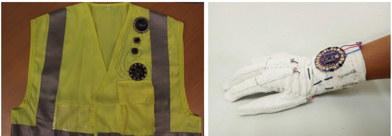
Fig. 4 (a) Safety vest for children, applying an Arduino LilyPad, from [48], originally published under a CC-BY-NC-ND license; (b) wireless smart glove, from [49], originally published under a CC-BY license.
