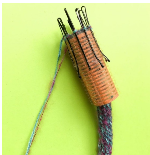
Figure 8. Circular knitting device created at home by one of the textile students.
