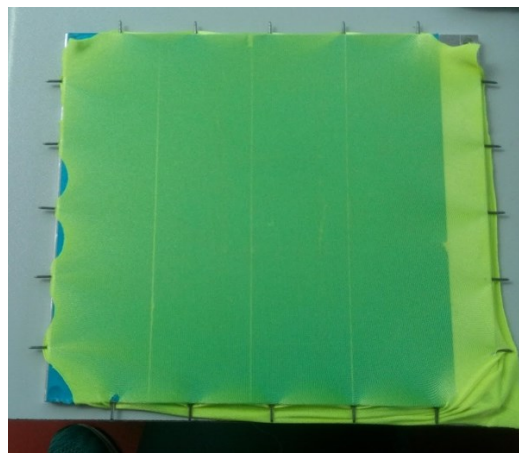
Fig. 7. Weft knitted fabric stretched and held in place on a plate prior to 3D printing. Pins at the edges of the plate hold the fabric still during the processing.
